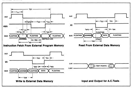
A.C. CHARACTERISTICS TA = 0°C to 70°C VCC = VDD = 5V ± 10%, VSS = 0V
